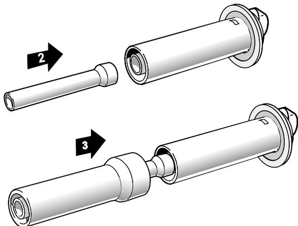
2. Fit the inner flue extension duct onto the inner flue duct.
