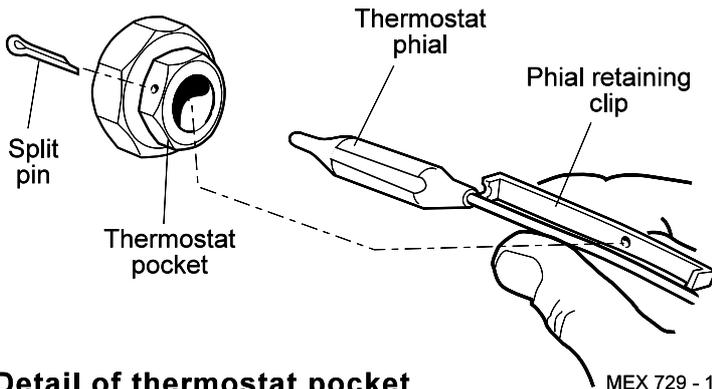
7. Insert the thermostat phial and phial retaining clip into the thermostat pocket. Take care not to kink the thermostat capillary as it is unwound and secure it with the split pin as shown.
