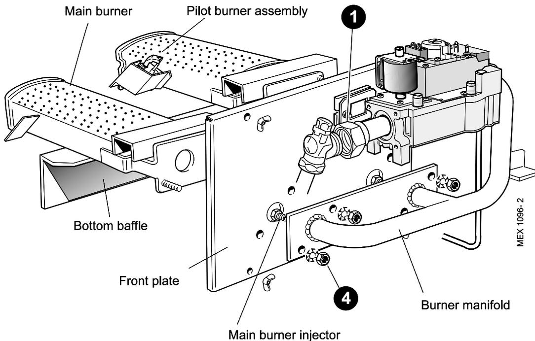
1. Remove the 2 screws and lift off the lower front panel then remove the grille assembly. Refer to Frame 57. Undo the gas cock union. Remove the 4 wing nuts and withdraw the burner and controls assembly, complete, from the boiler.
