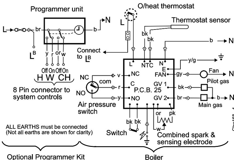
**Note.** If the optional Programmer Kit is to be fitted refer to the instructions provided with the kit and Frame 39.
