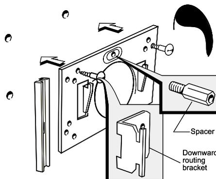
3. Fit the bottom 2 screws to secure the bracket(s) to the wall, through the wall mounting plate.
