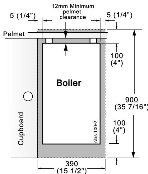
Front clearance: 533mm (17 3/4") from the front of the boiler casing.
