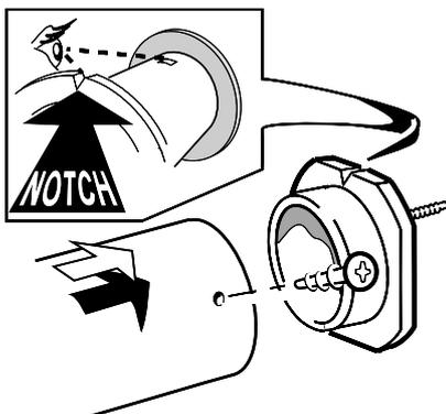
2. Drill 3 holes 3.2mm (1/8") dia. through the outer flue duct and boiler sealing ring. **Do NOT drill the inner flue duct.**
