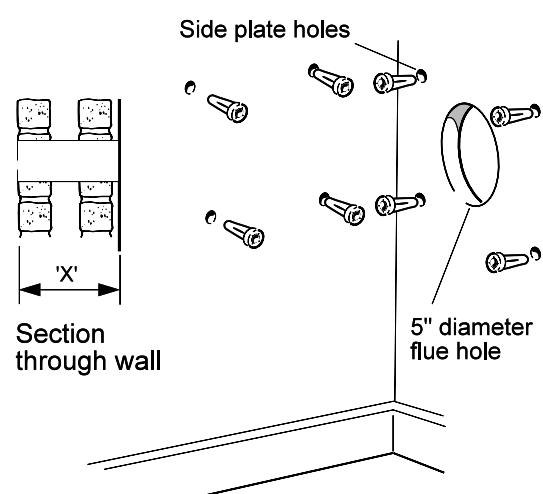
**Note.** If the terminal is to be sited within 25-40mm of a corner or vertical pipe (refer to Table 3) then the hole MUST be accurately cut and the rubber weather seal trimmed around the groove provided. The terminal wall plate need not be fitted.
