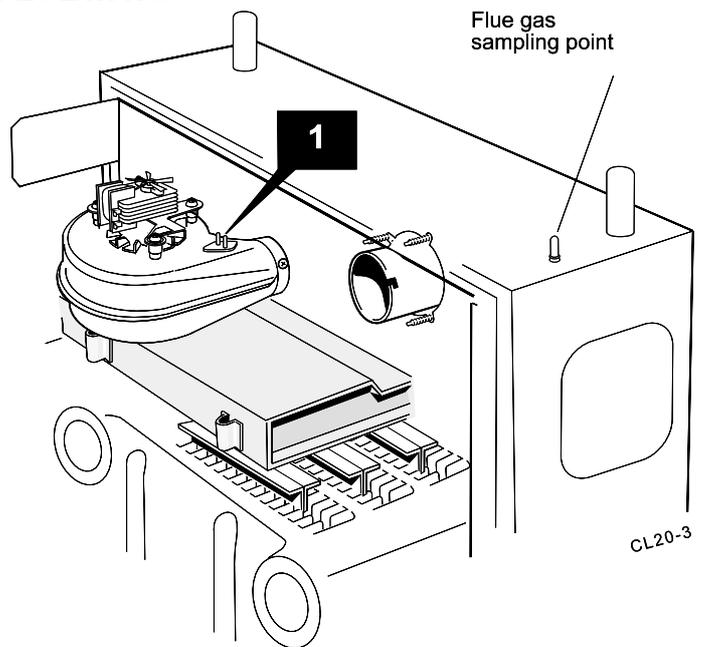
9. Remove all loose deposits from the heat exchanger, particularly between the fins, using a suitable brush.
