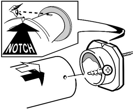
2. Drill 3 holes 3.2mm (1/8") dia. through the outer flue duct and boiler sealing ring. **Do NOT drill the inner flue duct.**
