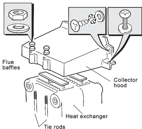
3. Uncouple and remove the flue baffles from the heat exchanger.
