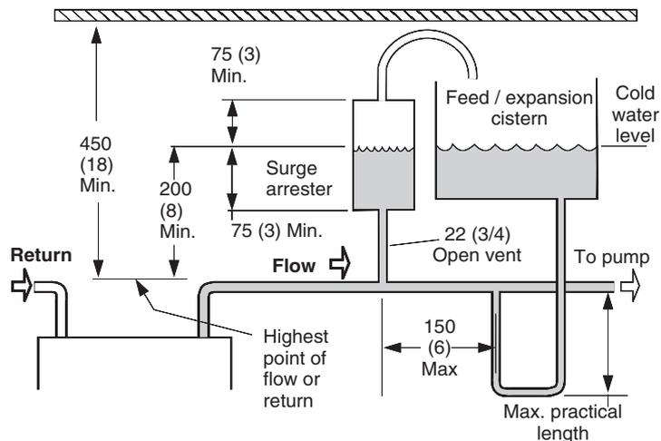
**Note.** The pump manufacturers minimum requirements must be complied with.
