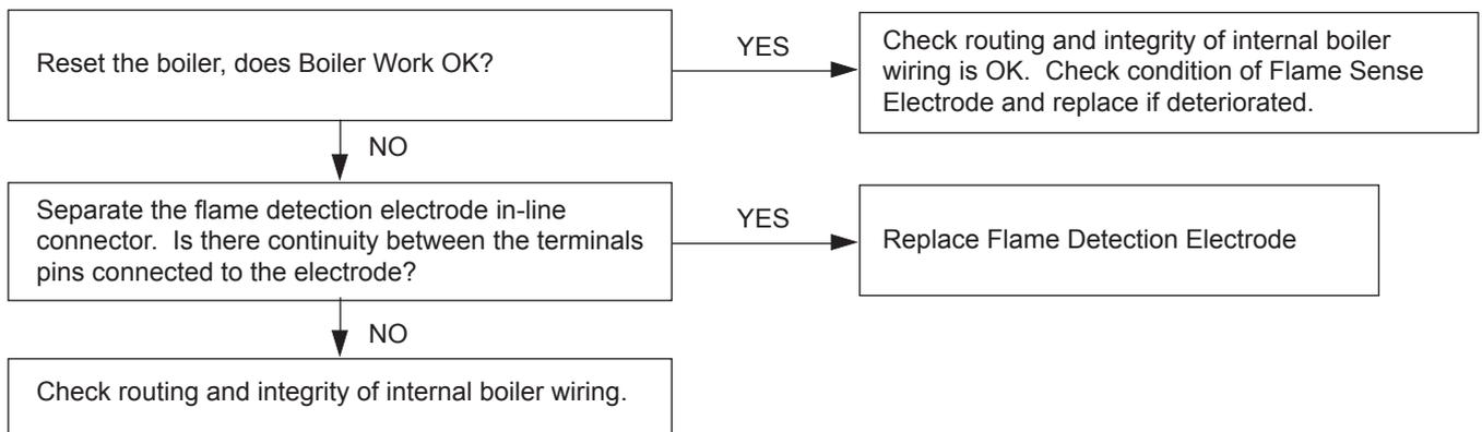
**RESET PROCEDURE** - To reset boiler, turn mode knob to reset position and immediately turn knob back to required setting.
