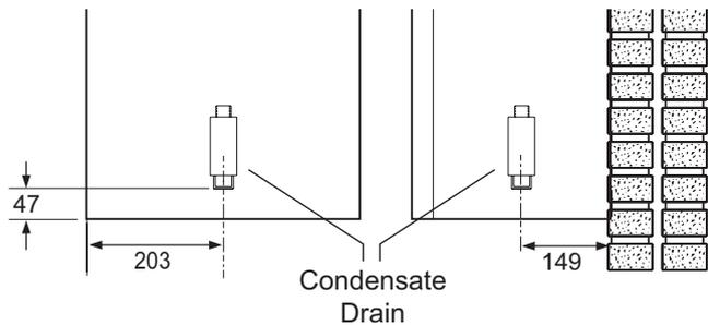
This appliance is fitted with a siphonic 75mm condensate trap system that requires filling before operating the appliance for the 1st time or after maintenance.
