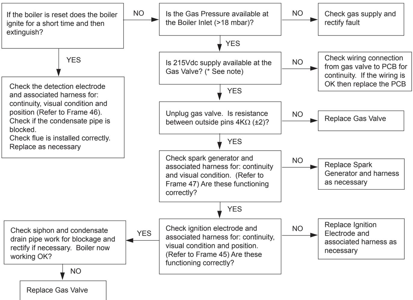
*\* Note: due to the wave form of the rectified voltage, the reading will vary depending on the type of meter used to measure the value. In general terms a reading greater than 150V indicates that the correct voltage is supplied to the gas valve.*
