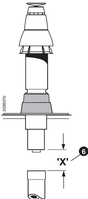
6. If the last extension duct requires cutting, measure 'X', the distance (outer ducts), between the duct and the terminal and add 100 mm to this dimension. This gives the length of the last extension duct.
