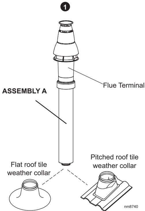
2. Fit the vertical connector (supplied separately) in accordance with the in the instructions provided with the vertical connector kit.
