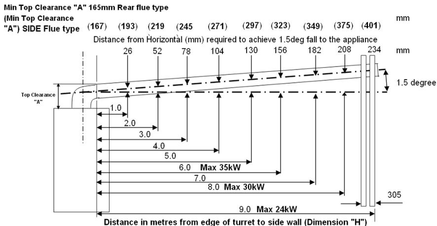
1. Dimension "H" must remain inside the Maximum flue length requirement for the designated output of the appliance been installed.
