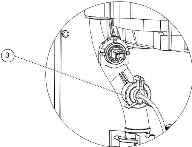
4. Releasing the two retaining clips on the pressure gauge ease the pressure gauge through the front of the control panel.
