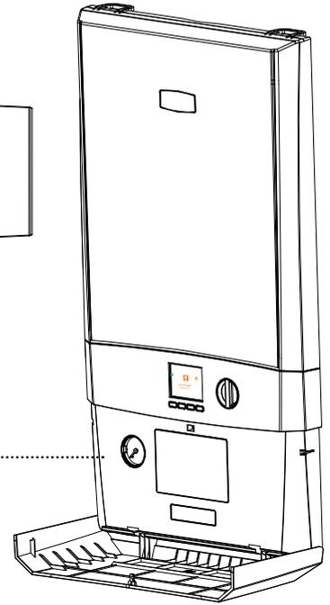
**CAUTION:** Do not operate the appliance before it has been fully vented of air. If it is necessary to operate the pump, do so with the gas service cock turned off.
