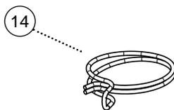
**! IMPORTANT** This clip needs to be fitted to ensure correct operation of the boiler.
