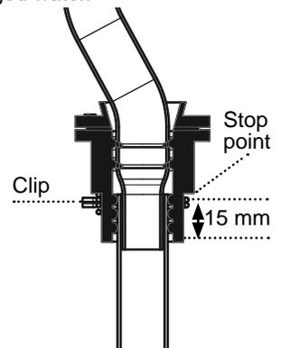
A purpose made PRV drain pipe is provided with the boiler to allow safe discharge through a wall to the outside of the building. This is particularly relevant to 'high rise' installations but can be used for all installations.
