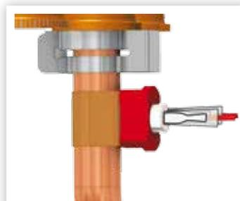
FIGURE 37. THERMISTOR SENSOR
