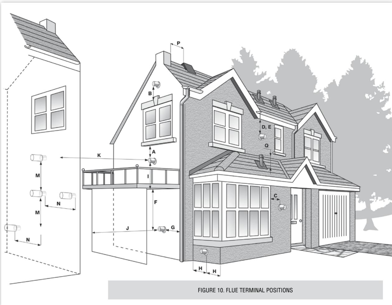
FIGURE 10. FLUE TERMINAL POSITIONS
