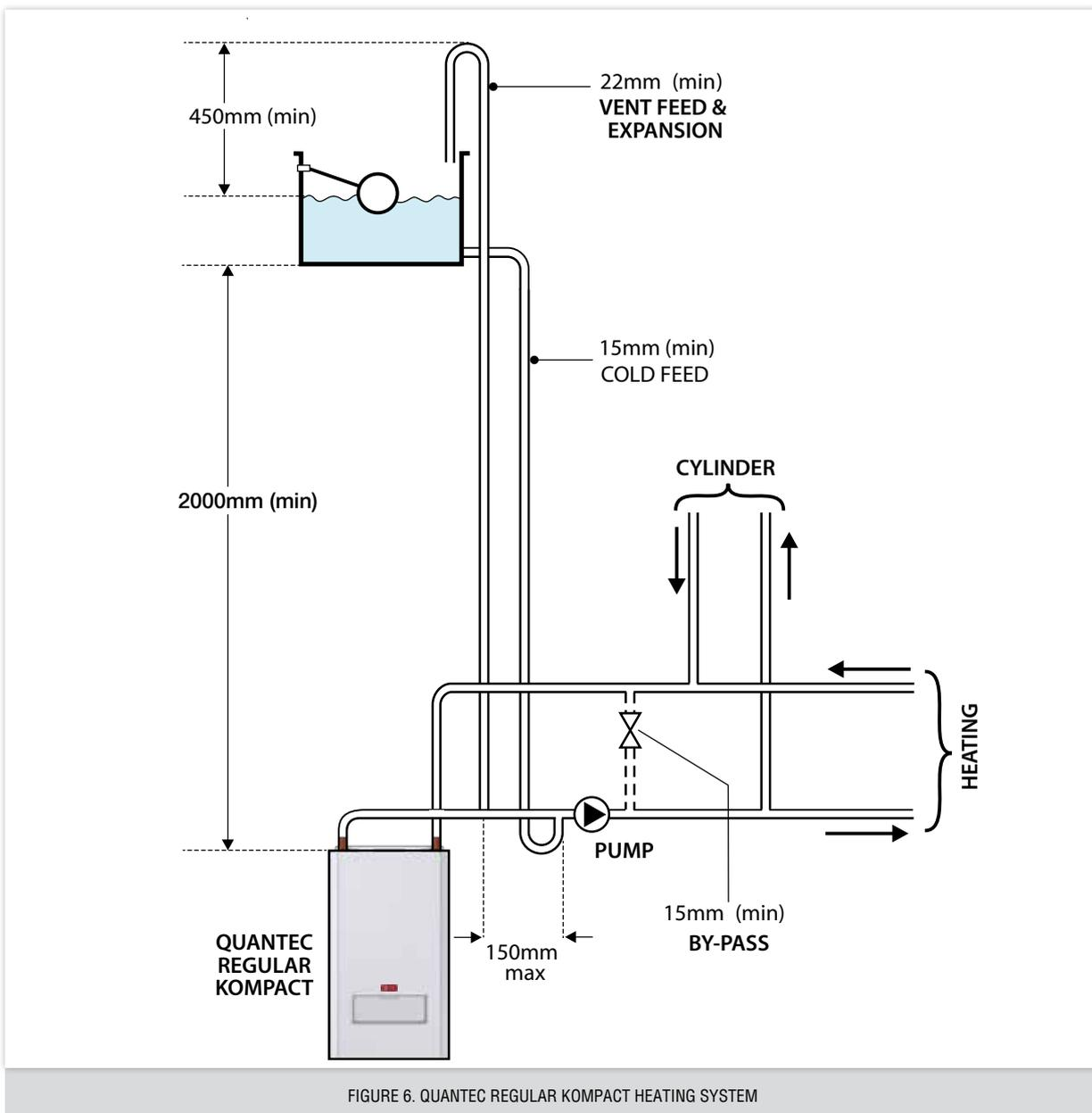
FIGURE 6. QUANTEC REGULAR KOMPACT HEATING SYSTEM
