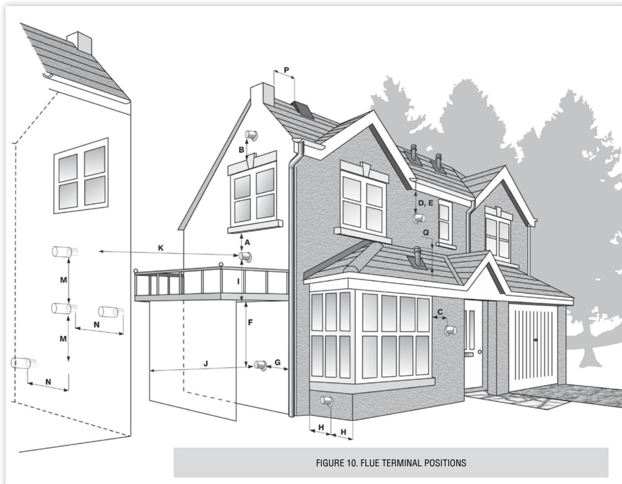
FIGURE 10. FLUE TERMINAL POSITIONS
