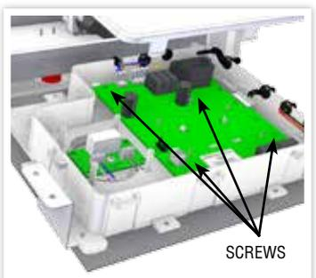
FIGURE 38. PCB ASSEMBLY
