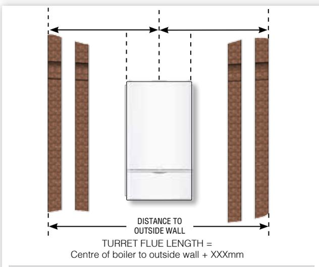
FIGURE 16. MEASURING WALL DISTANCES
