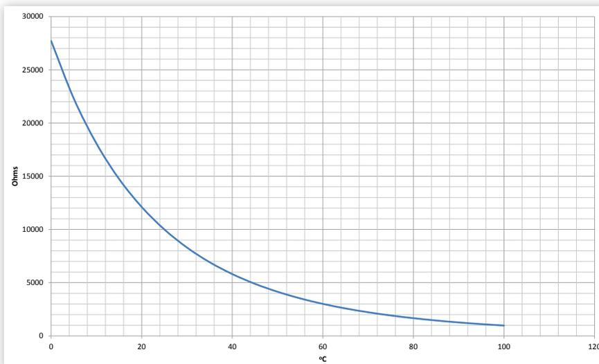
FIGURE 38. SENSOR TEMPERATURE/RESISTANCE DIAGRAM
