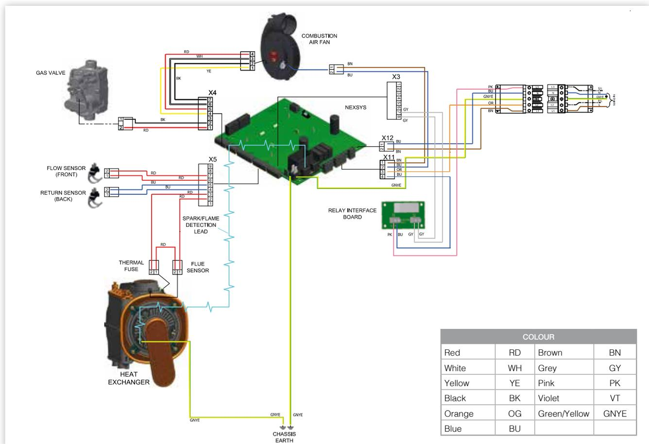
FIGURE 23. QUANTEQ REGULAR KOMPACT WIRING DIAGRAM
