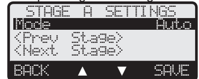
Sequencing Boiler Stage Menu
