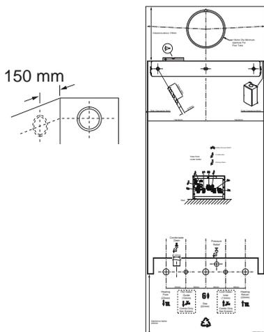
1. After considering the site requirements position the fixing template on the wall ensuring it is level both horizontally and vertically.
