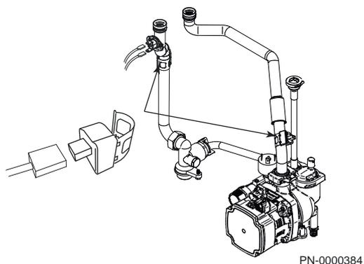
Fig.52 Removing safety overheat thermostat
