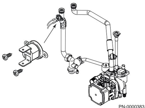
Fig.53 Remove safety pressure relief valve
