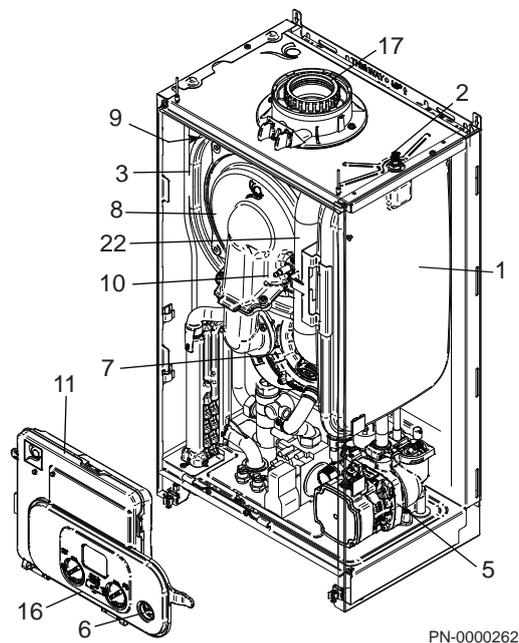
Fig.8 Hydraulic layout
