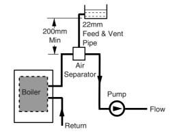
Fig. 10 Alternative Low Head Installation
