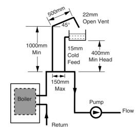
Fig. 8 Typical Low Head Installation
