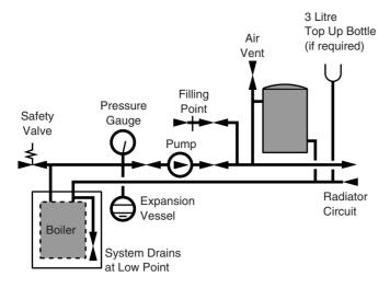
Max Boiler Flow Temp =  $82^{\circ}$  C Fig. 11
