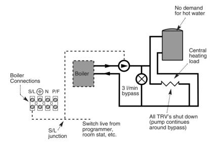
Fig. B Providing a 3 I/min bypass
