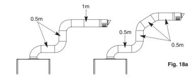
Pictorial examples of flue runs where EQUIVALENT flue length equals 4m
