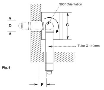
The 3° (1 in 20) fall provided by the elbow is to allow condensate to run back to the boiler, for disposal through the condensate discharge pipe.
