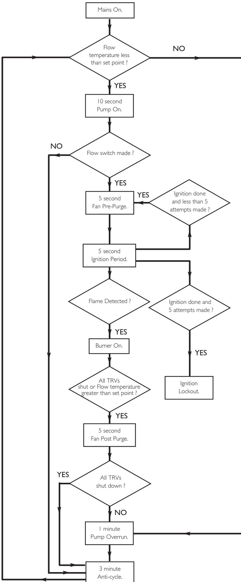
1. **Switched Live On:** When the switched live switches on if the flow temperature is less than the set point then pump overrun occurs. When the switched live switches on if the flow temperature is greater than the set point then pump overrun occurs.
