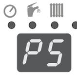
If the previous parameter “E” was confirmed by the **MODE** button, the display will show parameter “P” with value 0 to 9. Use buttons **-** **+** to shift the
