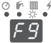
Under certain boiler parameters the customer or service settings may be lost – LED at symbol ☀ lights up. Switching the boiler off (wait about 10 seconds) and back
