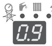
When the HeW pressure drops below 0.8 bar or rises above 2.5 bar, the LED at symbol
