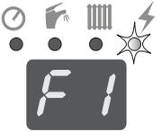
Flame loss due to interruption of gas supply to boiler – LED flashes at symbol ⚡. Switch the boiler off and after a while switch it back on using the main switch
