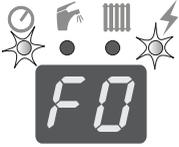
Loss of HeW pressure (under 0.6 bar) in the system. The boiler is automatically shut down – LEDs at symbols ⌚ and ⚡ are flashing. Add
