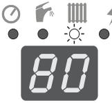
After turning the boiler on with the main switch, the current heating water temperature will appear on the display. LED at symbol
