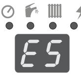
Press the **MODE** button repeatedly until the display shows the letter E with parameter 0 to 9. Use buttons **-** **+** to select the equithermal curve.
