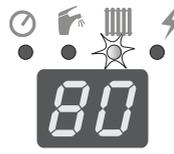
Press the **MODE** button repeatedly until the LED at the symbol
