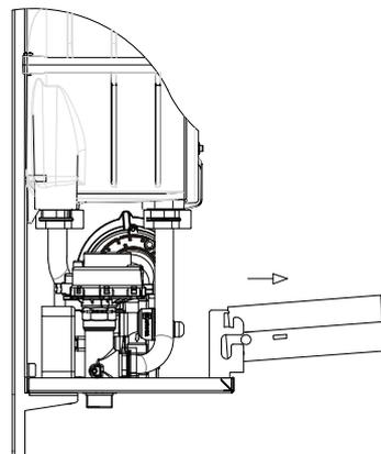
Unscrew the four screws the cover panel control box
