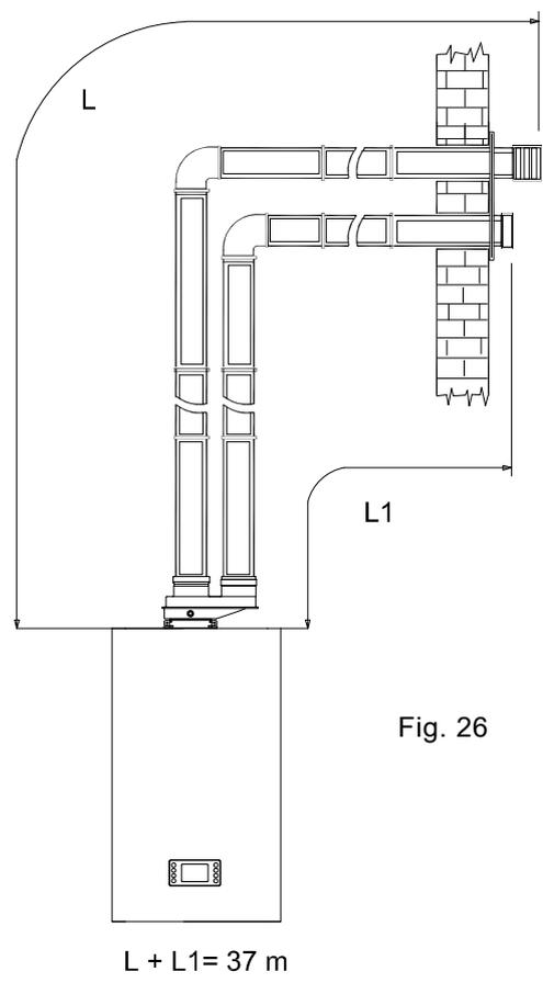
**5.16 Exhaust/suction system with concentric pipes for flat or sloping roofs. Extensions with two separate pipes (fig. 24).**
