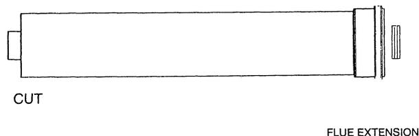
Starting at the appliance end, assemble the extension duct sections, making each inner and outer (flue) joint by inserting the spigot end into the socket end of the next tube, making sure the seal rings are correctly located (Fig. 44). Make sure that the entire flue is adequately supported. Use at least one bracket for each extension used.
