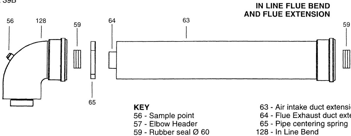
**5.7.2** Positioning the elbow towards the required direction (Fig. 30).
