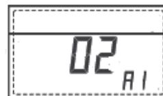
Use the and buttons to set the number of boilers in the cascade.
