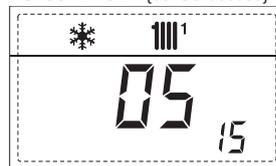
17. Display of D.H.W. flowmeter load (i.e. 18 l/min and 0.3 l/min) or flow switch [respectively ON and OFF]. Combi boiler only.
