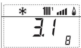
9. Display fan speed in rpm x 100 (e.g. 4.800 and 1850 rpm)
