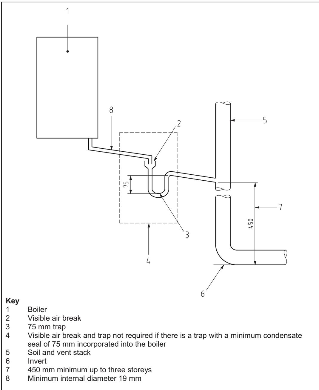
**Figure 2(a) – Connection of a condensate drainage pipe downstream of a sink, basin, bath or shower waste trap**
