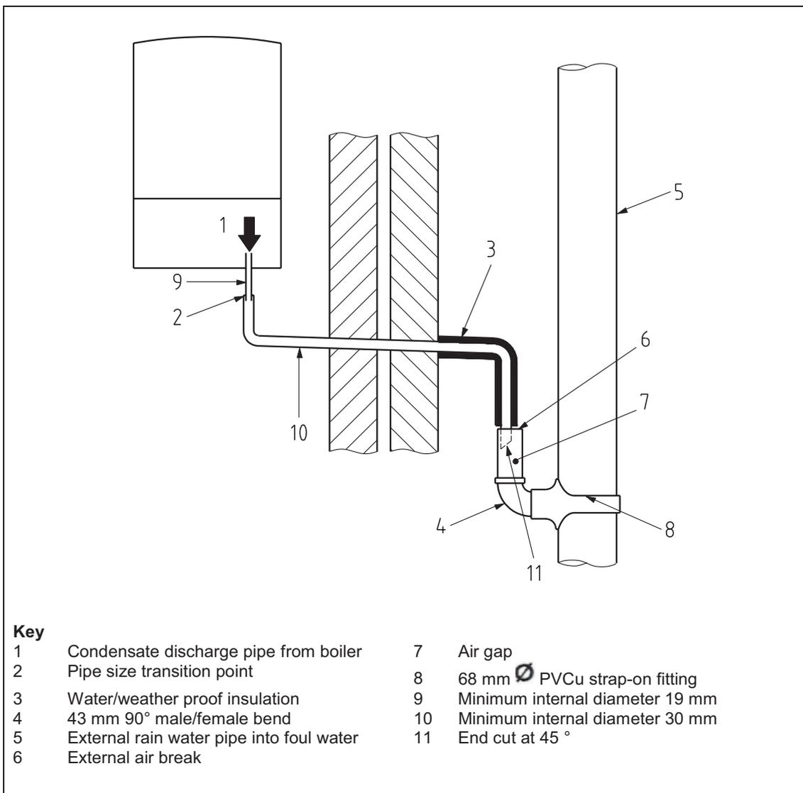
Figure 6 – External drain, gully or rainwater hopper
