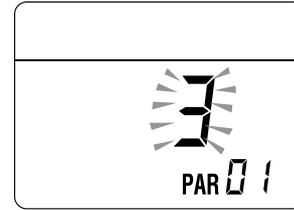
When all the parameter modifications have been made, exit the parameter menu by pressing and holding down the buttons and all at the same time for at least 5 seconds until the initial screen is displayed.
