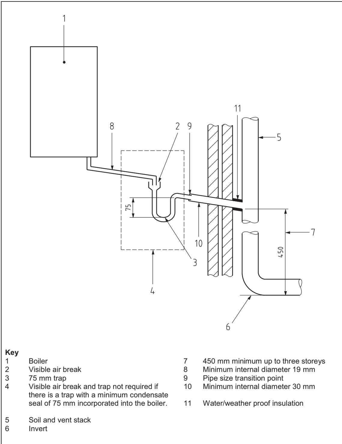
Figure 5 – External termination to rainwater downpipe (NB only combined foul/rainwater drain)
