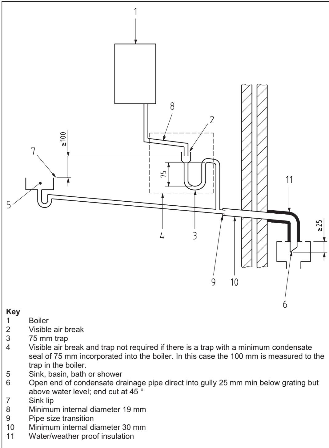
Figure 2(b) – Connection of a condensate drainage pipe upstream of a sink, basin, bath or shower waste trap
