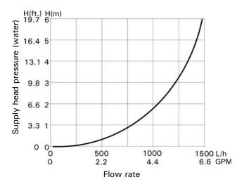
Boiler maximum flow rate 6.2 GPM (1400 L/h)
