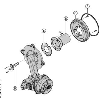
Check the burner gasket (A) and burner cylinder assembly (D) for damage and replace if necessary. Replace the cylinder burner assembly if damaged.
