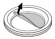
When utilizing the combustion air inlet cover (A) for Vitodens 100-W series boilers, remove the center section and leave the rubber seal in place.
