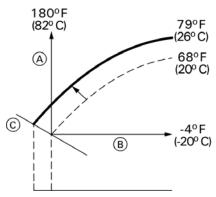
Adjustment of the increase set point temperature from 68 to  $79^{\circ}F$  (20 to  $26^{\circ}C$ )
