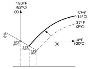
Adjustment of the reduced set point temperature from 37 to  $52^{\circ}F$  (3 to  $14^{\circ}C$ )
