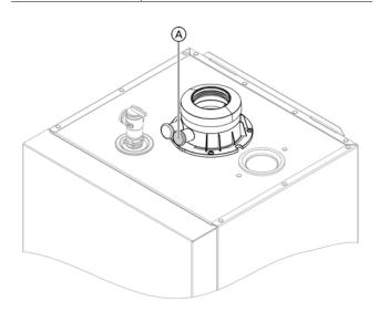
A Flue gas measuring port
