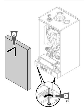
To ensure continued efficient operation of the boiler, it is recommended that it is checked and serviced as necessary at regular intervals. The frequency of servicing will depend on the particular installation conditions and usage but in general once a year should be adequate. Any service work must be carried out by a licensed professional heating contractor.
