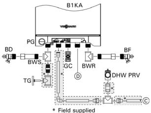
**Note:** The B1HA DHW supply and return connections are supplied capped. For installations that require DHW tank connections remove caps. For installations that do not require DHW tank connections leave caps installed.
