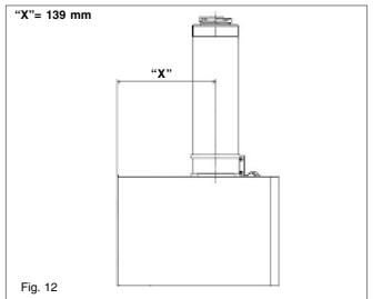
Fit the appropriate flashing plate to the roof and insert the vertical flue terminal through the flashing plate from the outside, ensuring that the collar on the flue terminal fits over the flashing.
