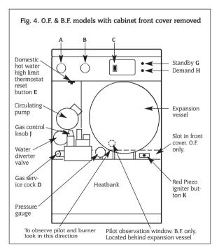
dow **L** (BF) or under the combustion chamber door baffle (OF). When the pilot lights, continue to hold the grey gas control knob in for a further 15 seconds and then slowly release it.
