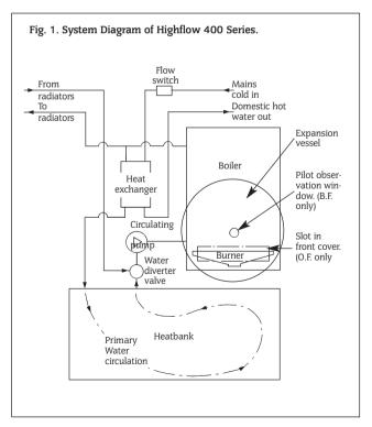
When domestic hot water is no longer required the burner and pump will continue to operate until the heatbank is back to the required temperature.
